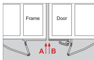
With the door closed, take the **Wide** strip and peel off the tape backing.
