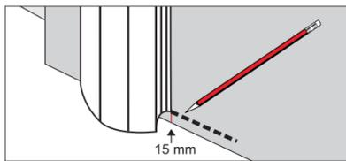
On both the door and the door frame, use a soft pencil to draw a horizontal line approximately 0.6" (15mm) from the bottom of the door. Make this mark on both the "Push" and "Pull" sides
