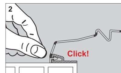
Insert the loose side of the **Wide** strip and insert into the **Click** strip.
