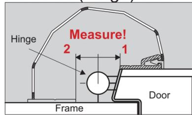
Measure the distance between the center line of the hinge and the edge of the rabbeted door (1). Use this same measurement to mark an equal distance on the frame from the center of the hinge (2).
